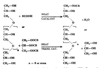
FIG. 4. Synthesis of polyglycerol partial ester (23). R may be saturated or unsaturated, aliphatic or aromatic, monocarboxylic or di-, and polycarboxylic may form mono- or polyester.
