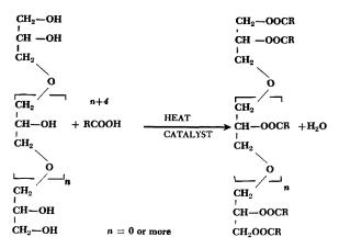
FIG. 5. Synthesis of polyglycerol complete ester (23). R may be saturated or unsaturated, aliphatic or aromatic, or one or more fatty acids.
